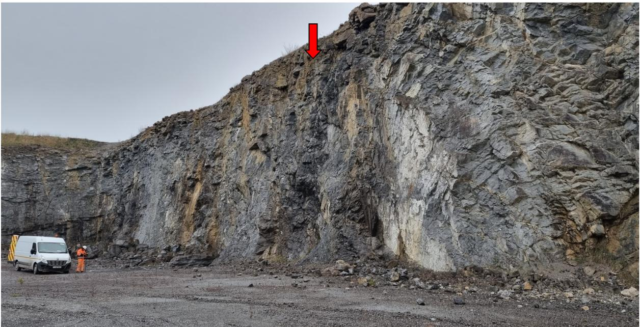
*Fig. 4.2 Looking north at northeast face in northwest extension area. Interpreted fault location is shown by arrow.*
